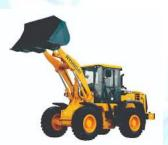
the loader toward and into piles of snow in order to fill the front scoop or bucket. The operator then lifts the bucket, drives the loader to the snow dump zone, and then dumps the snow. The truck is large enough so that the operator of the front loader can dump the contents onto a pile 14 feet high. This allows the operator to create massive piles of snow.
